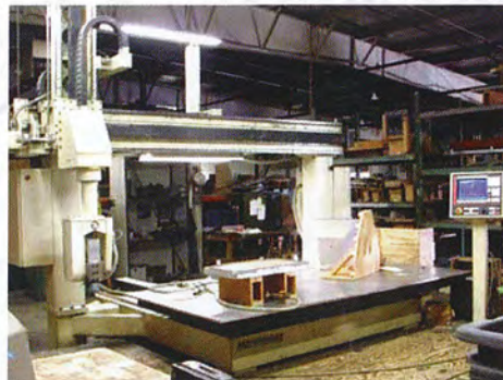
CNC Trim Station
